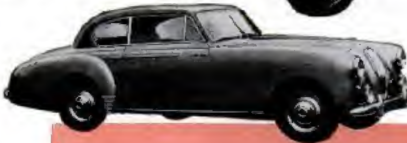
LAGONDA , below, is among the world's most advanced cars, with independent suspension on four wheels, inboard rear brake drums, built-in jacks and an entirely flat floor. It has six cylinders
